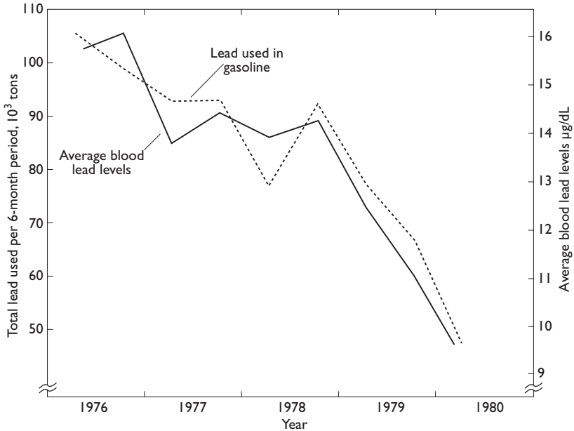
FIGURE 6. Blood lead levels decline dramatically with reduction of lead in gas, 1976–1980. Declining blood lead levels continued to today following the complete removal of lead from gasoline and improved abatement techniques. Source: U.S. EPA, Air Quality Criteria for Lead , vol. 3, EPA-600/8-83/028cF (Washington, D.C.: U.S. EPA, June 1986), 11–43. See also David Jacobs, “Environmental Health Disparities in Housing,” AJPH , 1012 (Supplement 1, 2011), p. S117.
